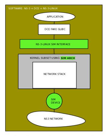
The green parts are implemented in ns-3-linux source files, the grays parts comes from the Linux kernel sources and are not modified at all or with only few changes. Application should not be modified at all.
