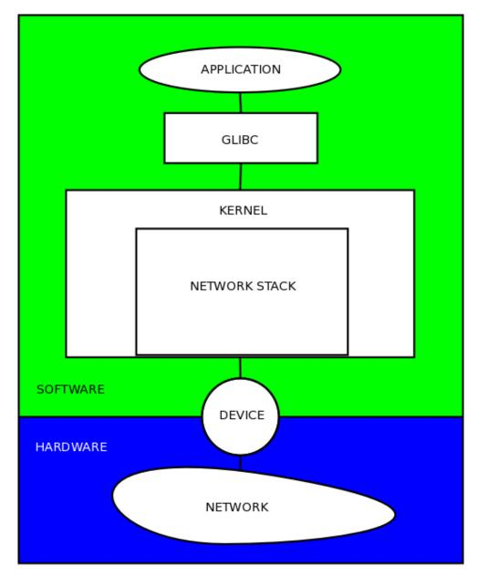
The following schema show the same application running under DCE and *ns-3* and using a real kernel network stack:
